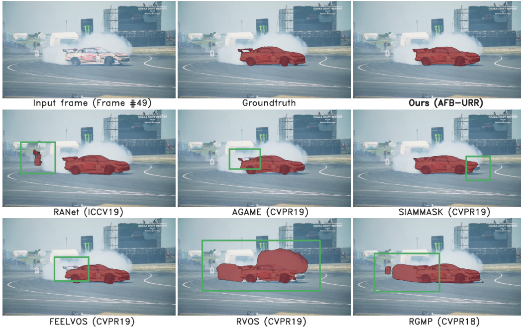
Figure 2: Qualitative results of the test video drift-chicane from the DAVIS 17 dataset. We show the segmentation on a challenging frame (frame #49) where the car is surrounded by smoke.
