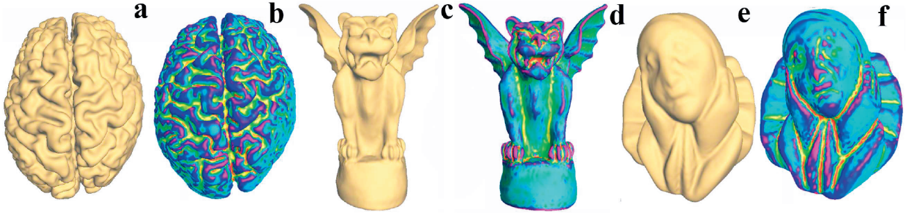
Fig. 7. Examples of degree-4 spherical DCB-splines. From left to right: the fitted spline surfaces followed with mean curvature distribution: Brain, Gargoyle, and Pierrot. Their maximum fitting error/root mean square error are: Brain (0.493%/0.090%), Gargoyle (0.636%/0.065%), and Pierrot (0.574%/0.058%).
