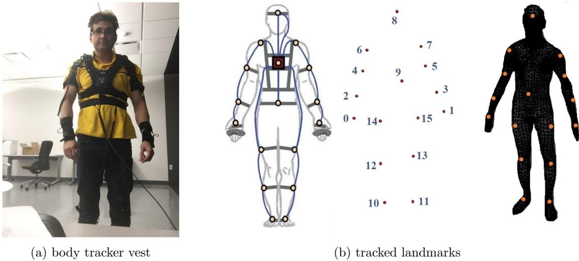
Fig.3. A wearable body tracker vest is used to track feature landmarks on human body (a). 16 corresponding feature points are extracted on the human body mesh template.
