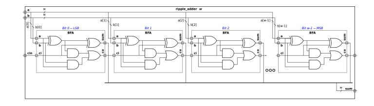
(c) If cin were removed (or set to zero) the cost and delay of the optimized adder would depend on a. Explain why, and illustrate with the example of a=2.
