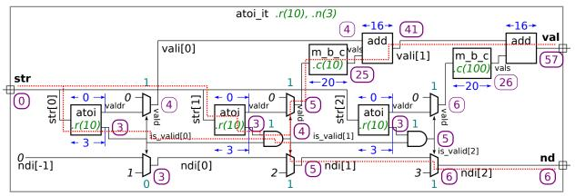
(b) Modify the design to reduce the delay at val by moving multiplexors. The modification is simple though will increase cost. Show your modification either on the diagram or in the Verilog code below.
