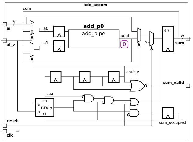
Show the timing (signal arrival time at each component output) and  $\Box$  the critical path.  $\Box$  Note that aout arrives at t = 0.
