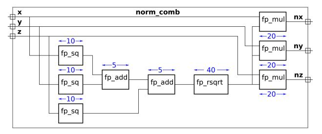
(a) Compute the latency and throughput norm\_comb given the timings shown in the diagram.
