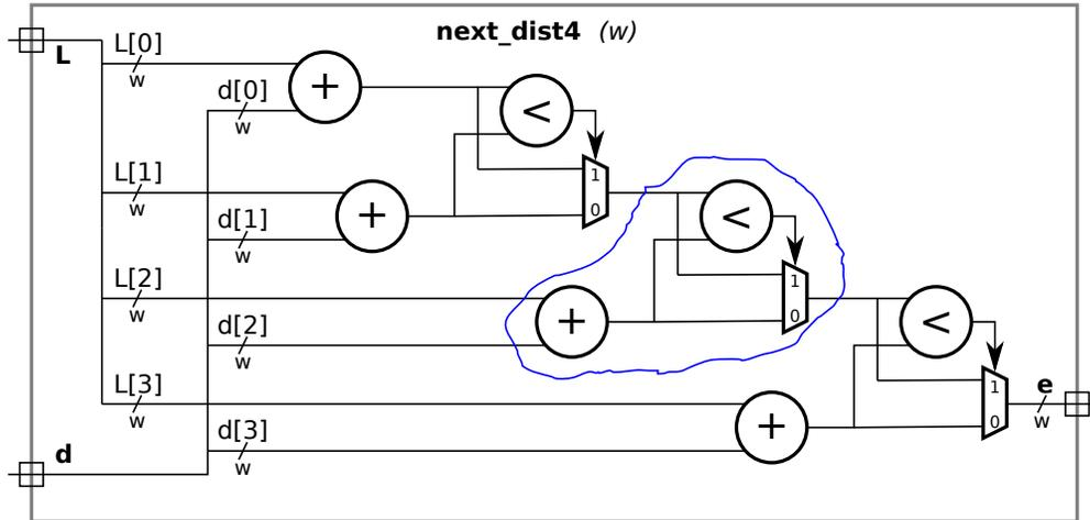
(a) Compute the cost and delay of the module using the simple model, and show the critical path on the illustration. Assume that the adder and comparison units are based on ripple adders.
