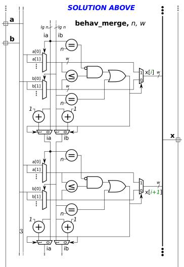
Problem 2: [20 pts] Appearing once again is part of the Homework 6 solution, this time with items labeled in blue. Show the cost and delay of these, as requested below. See the previous problem for the Verilog description. The phrase *most expensive* means for the value of i for which the device needs all inputs, even after optimization. For the mux, show the cost and delay for the tree implementation.
