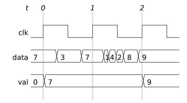
Inference of Registers > Coding Common Edge-Triggered Registers > With Enable
