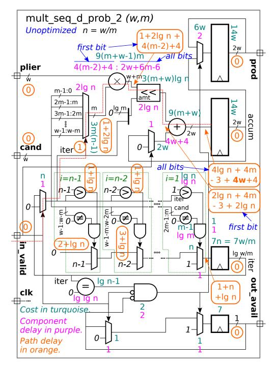
The costs and delay of each component are shown in the diagram above. The path delay for selected paths is shown in the circled orange numbers. Note that one input to all of the comparison units (for example, the zero in  $\neq 0$ ), is a constant, reducing their costs and delays. Many of the multiplexors also have one constant data input.
