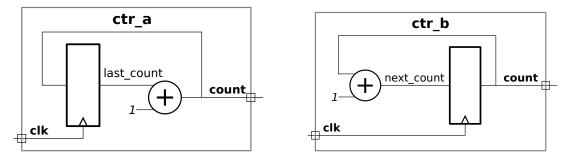
(b) There is a big difference in the timing of the outputs of ctr\_a and ctr\_b. Explain the difference and illustrate with a timing diagram.
