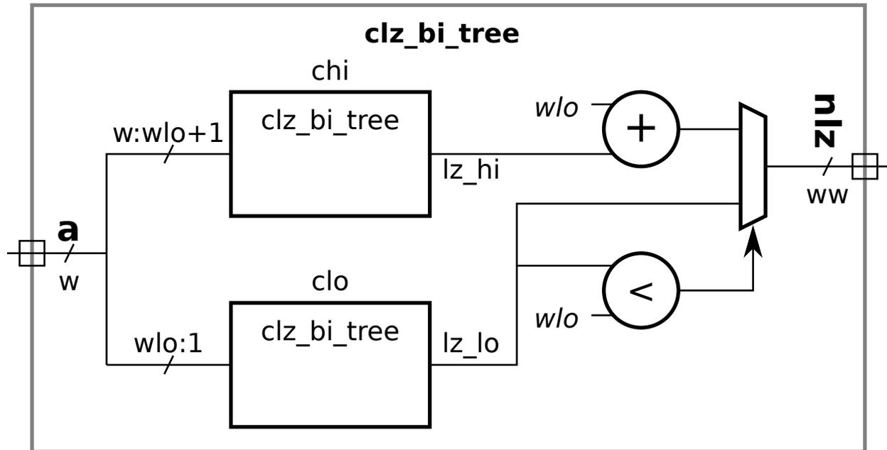
Problem 2: [25 pts] In Homework 2 a `clz` (count leading zeros) module was constructed recursively by splitting the input bit vector and connecting each half to a smaller instance. The incomplete module below is similar except that the input vector is to be split into thirds and each third connected to a recursive instance. Complete the module.
