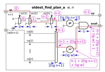
Plan B:  $\bigvee$  show delay along all paths,  $\bigvee$  highlight the critical path,  $\bigvee$  and show the delay through each component. Show these  $\bigvee$  in terms of w and n, and  $\bigvee$  account for constant inputs such as the zeros in the equality units.
