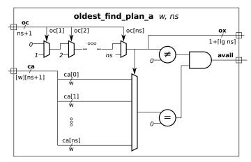
The  $\neq 0$  unit can be realized using a  $\lceil \lg n \rceil$ -input OR gate, and the = 0 unit can be realized using a w-input NOR gate. The costs are the number of inputs minus one. The total cost is:
