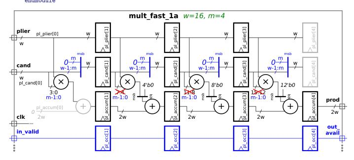
Solution appears above in blue. A straightforward addition is the pipeline latch,  $pl_{occ}$ , to pass the  $in_valid$  signal. The other change is in the way that the multiplicand is passed from stage to stage. In the original design the multiplicand (cand) was passed
