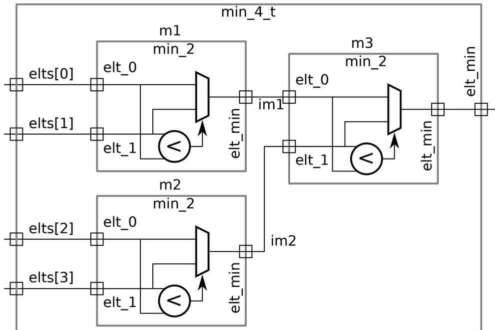
(b) Draw a diagram of the hardware that will be synthesized for the `min_4_1` module below. Your diagram should include two-input multiplexers and a comparison module.
