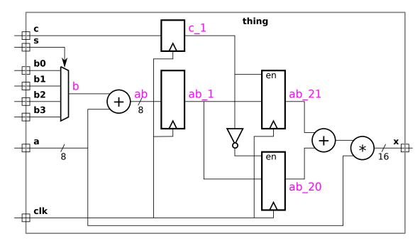
The solution appears below. Names for wires that were unlabeled in the problem appear in purple. (That is, the purple labels are part of the solution.) Note the use of case/endcase for the mux. Though using an if/else chain or the conditional operator, ?:, would be correct, they are more tedious and prone to error and so it's worth taking the trouble to remember to use case.
