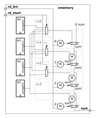
(b) Appearing below is Plan B for the module. Though we know it produces the same value for sum as Plan A, it might be synthesized into different hardware. Show the hardware synthesized for Plan B.
