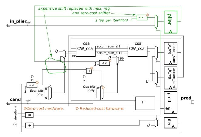
(d) Explain how the streamlined multiplier described in class eliminated the plier shifter without having to add a register.
