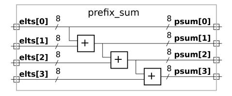
(b) Estimate the delay for the synthesized hardware before optimization. Use w for the value of wid and L for len. Assume that a w-bit adder has delay w.
