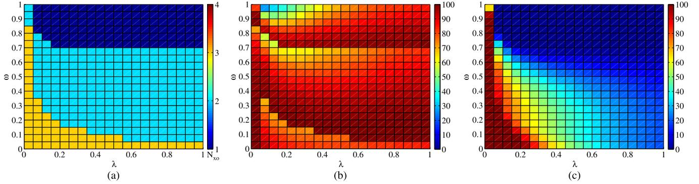
Fig. 5. Numerical results with CRP ( $s = 10$ ,  $N = 5$ , and  $M = 10$ ). (a) Channel allocation map. (b) %age collision in total loss. (c) %age loss increment for  $N_x = 1$  w.r.t. optimal.
