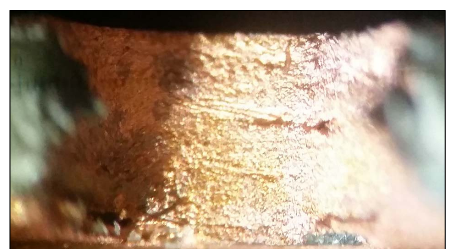
10x image of copper coated via
