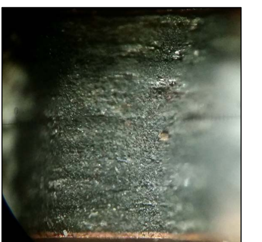
10x image of via coated in activator
