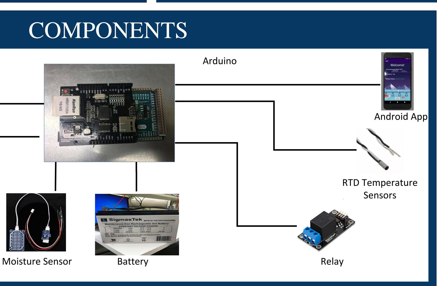
N – 8VDC in from the power supply V – 5V pin to power sensing circuits V – 3V pin to power moisture circuit Input/Output pins for sensing ircuits, heater control, and erro
