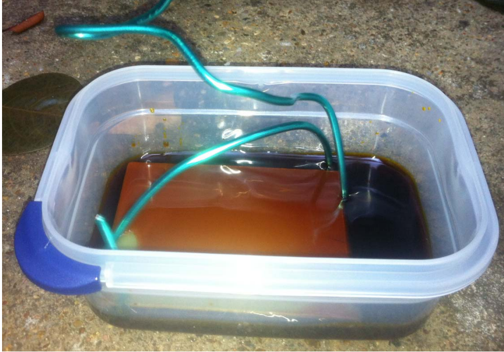
Figure 26 – PCB immersed in Etching Solution
