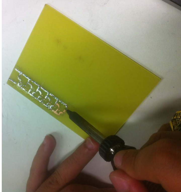
Figure 28 – Soldering the Circuit
