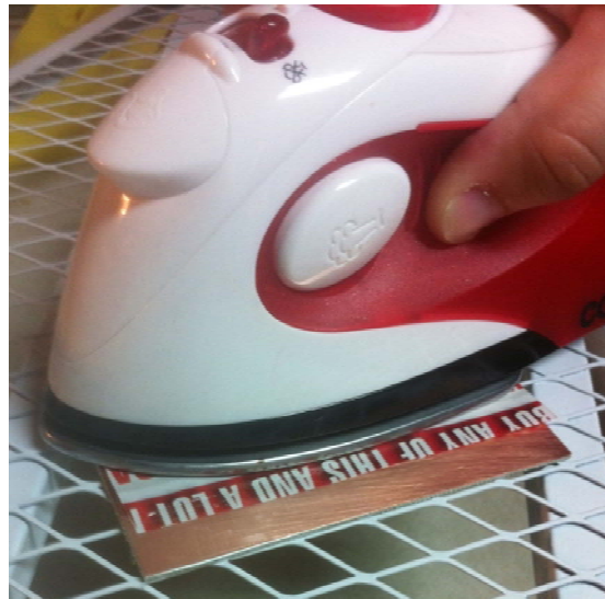
Figure 23 – Heat Transfer Process
