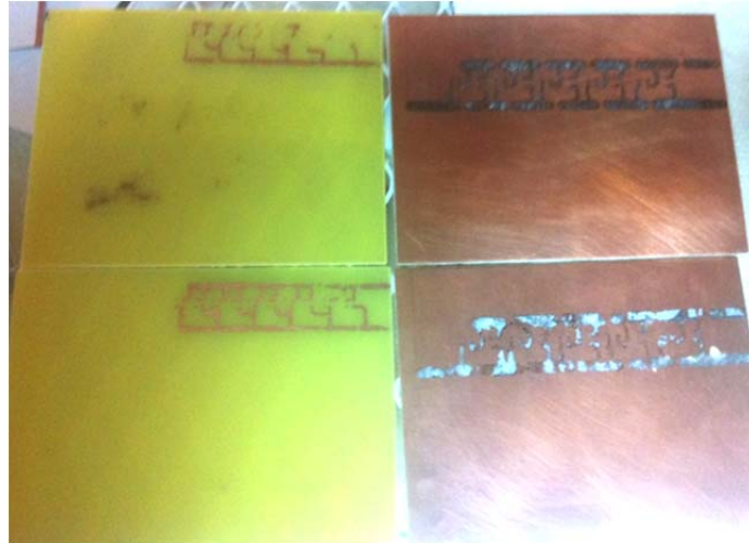
Figure 27 – Fully Etched PCBs next to Un-Etched PCBs
