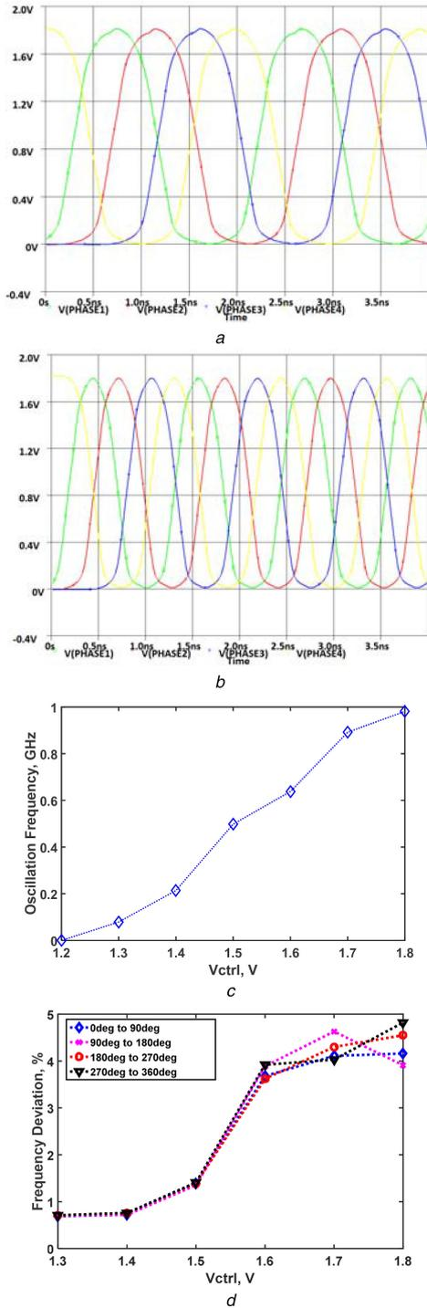
**Fig. 6** Simulations of clock generator
