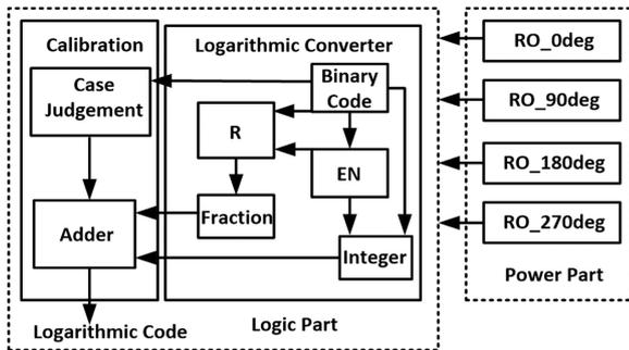
**Fig. 3** Block diagram of the proposed logarithmic converter
