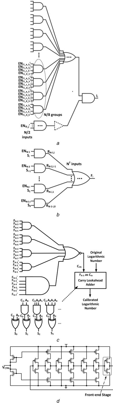
**Fig. 4** Circuit diagram of the proposed  $N$ -bit logarithmic converter (a) Integer part, (b) Fraction part, (c) Calibration block, (d) Clock generator
