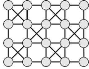
Fig. 2. Standard Mesh Network for Superconducting Quantum Computer
