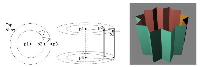
(b) Appearing below again is the code from the Homework 2 solution. This time the goal is to render a (crude) gear positioned and oriented using the same four points, p1-p4. The points define two pairs of circles as illustrated above. The center illustration shows how one tooth (gear part) is constructed. There should be n\_pieces teeth, positioned so they touch and go around the gear as shown on the screenshot to the right. Modify the code to draw the gear.
