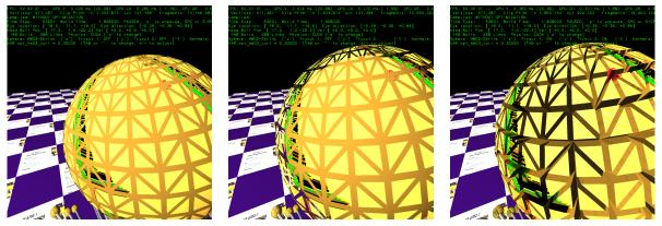
The new faces are formed using vertices of the original triangle and the shrunken one. (There is no need to render the original triangle.) The new faces should use a darker color and texture coordinates should be applied so that it appears that whatever texture color appears at a point on the edge of the shrunken triangle is used on the path down toward the sphere surface. See the screenshot. (This is an easy thing to do.)
