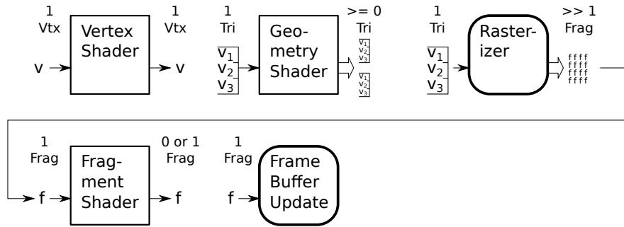
(a) The diagram shows 16 f's at the output of the rasterizer stage, but that's not necessarily the actual number.
