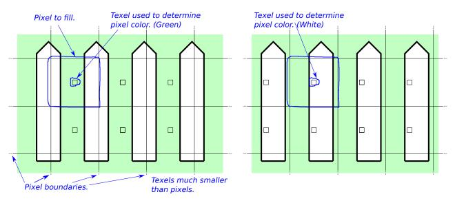
(b) Re-draw the diagram showing how the choice of an appropriate MIPMAP level can avoid the problem of the fence disappearing.
