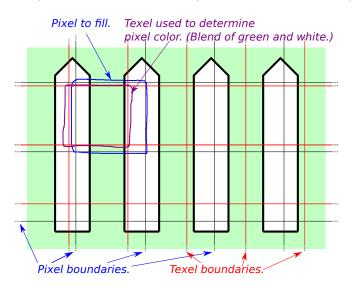
(c) Draw a diagram showing an example of how linear filtering can improve the appearance of the fence.
