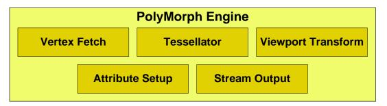
The first stage begins by fetching vertices from a global vertex buffer. Fetched vertices are sent to the SM for vertex shading and hull shading. In these two stages vertices are transformed from object space to world space, and parameters required for tessellation (such as tessellation factor) are calculated. The tessellation factors (or LODs) are sent to the Tessellator.
