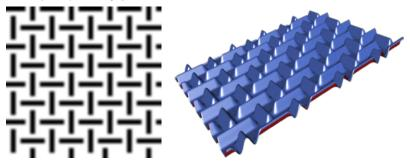
When a displacement map (left) is applied to a flat surface, the resulting surface (right) expresses the height information encoded in the displacement map.
