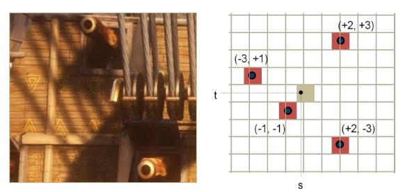
The soft shadows in 3DMark 2006 (left) are implemented through jittered sampling of a texture map (right). GF100 implements jittered sampling in hardware, delivering up to 2x the performance of GT200.
