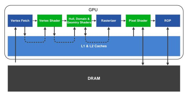
GF100's cache architecture enables efficient communication between pipeline stages and reduces off-chip memory traffic.
