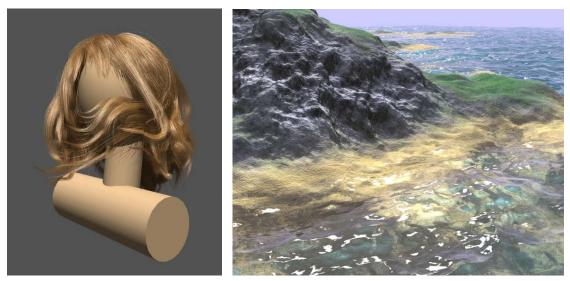
The Hair demo (left) uses tessellation, geometry shaders, and physical simulations. The Water demo (right) uses tessellation in large environments.
