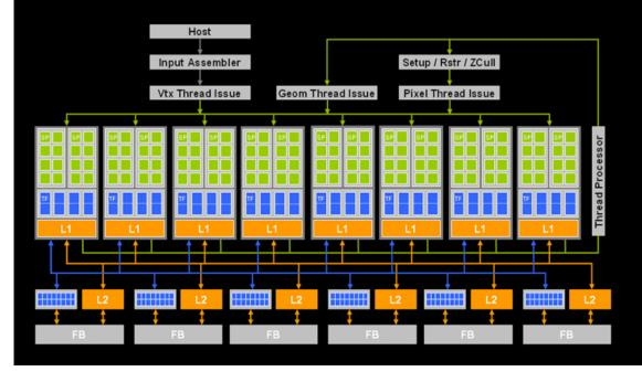
Figure 26. GeForce 8800 GTX block diagram
