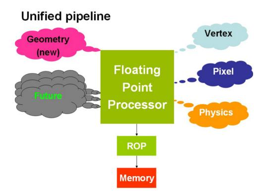
Figure 17. Conceptual unified shader execution framework
