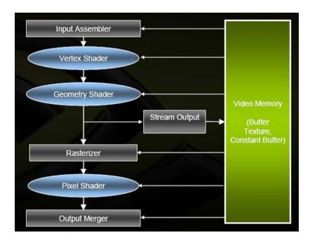
Figure 28. Direct3D 10 pipeline
