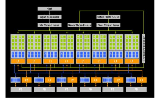
Figure 12. GeForce 8800 GTX block diagram
