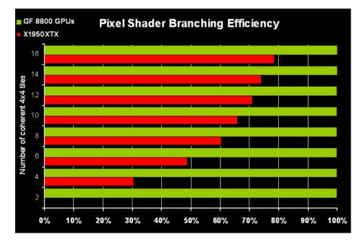
Figure 23. GeForce 8800 GPU pixel shader branching efficiency
