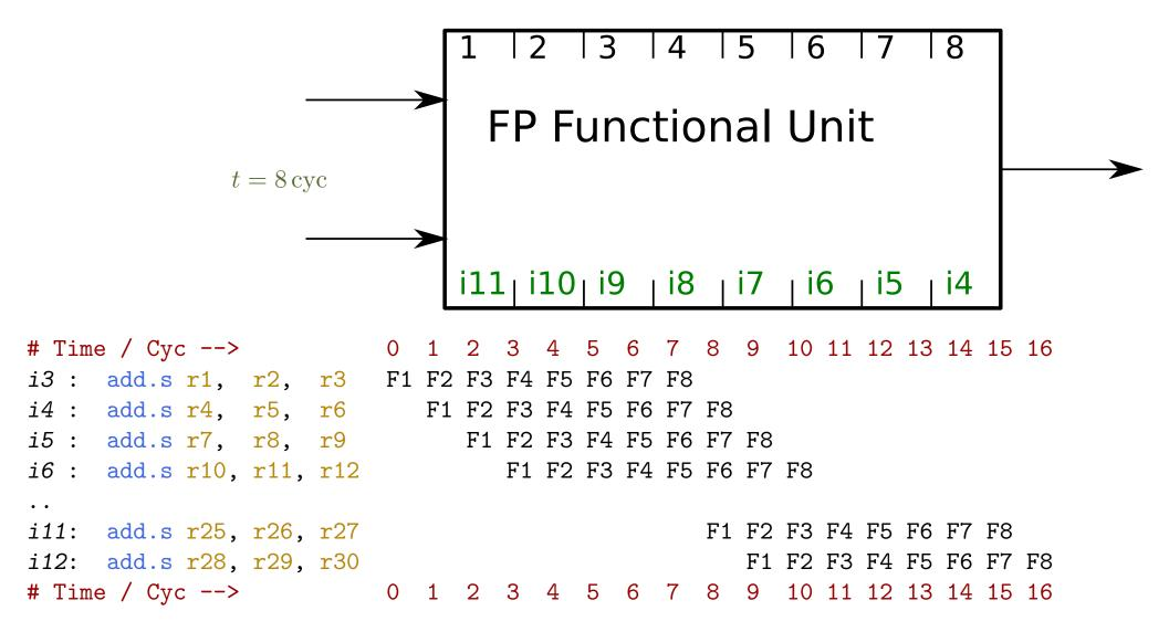
Pipelined Floating-Point Functional Unit >> Bandwidth and Throughput
