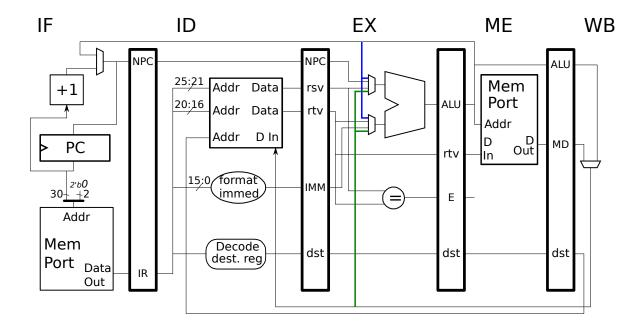
Blue bypass used in cycle 3, green bypass used in cycle 4.
