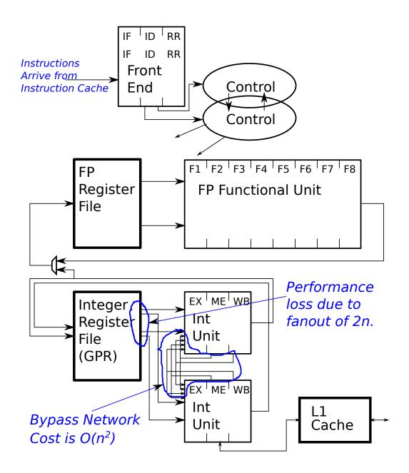
Superscalar Cores  $\gg$  Typical Superscalar Cores
