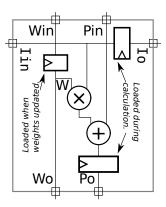
Illustrated below is an array of  $4 \times 4$  mac units, with inputs partially labeled. Connections are shown for the inputs and partial sums, but not for the weights. The array is used to compute O[n][x] += I[n][i] \* W[i][x].
