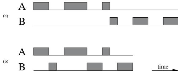
Figure 1: If two parallel libraries, *A* and *B*, execute one after the other, as in (a), the libraries’ idle times are not hidden. Interleaved execution, as in (b), is more efficient and happens automatically in a data-driven system.
