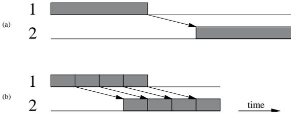
Figure 2: Coarse-grain computations lead to large communication latencies, as shown in the two-processor utilization diagram in part (a). Fine-grain computations, as in (b), allow communication to be pipelined, increasing processor utilization and decreasing the impact of network latency on performance.
