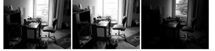
Fig. 4. Images of the same scene captured with a Canon G5 digital camera. These are three of the 15 images used in restoration. The highest exposure time is 1/50 s, and the lowest is 1/800 s.
