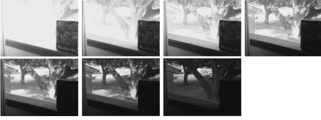
Fig. 3. Images of the same scene captured with a Canon G5 digital camera. The exposure times are 1/25, 1/50, 1/100, 1/200, 1/400, 1/800, and 1/1250 s.
