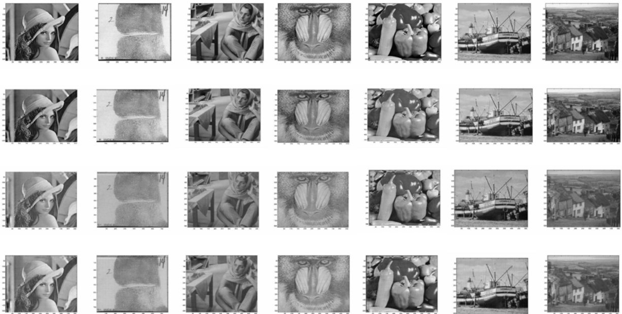
Figure 10. Comparison of standard image sequences using WSQ (rows from top to bottom): originals, Cohen-Debauchies-Feauveau single stage floating point, CKB 9/7 3-stage integer, TAY 9/7 3-stage integer.
