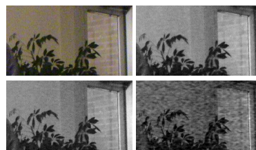
Fig. 1. Portion of an image captured with a Sony DCR-TRV27; and its red, green, and blue channels. The blue channel is the most degraded channel. The noise apparently has low- and high-frequency components.
