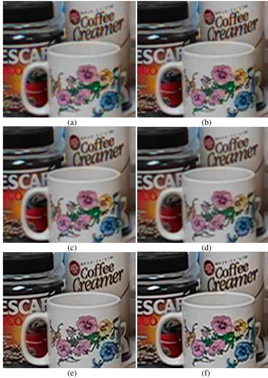
Fig. 5. Single- and multi-frame demosaicking results. (a) Single frame demosaicking using [3]. (b) Single frame demosaicking using [7]. (c) Multi-frame demosaicking with detail and observation constraints used ( T_d=1 , T_o=20 ). (d) Multi-frame demosaicking with all constraints applied ( T_d=1 , T_o=20 , \tau_S=4 , \tau_I=6 , T_c=2 ). The iteration number for multi-frame demosaicking is five. (e) Sequential SR result using images multi-frame demosaicking with all constraint sets. (f) Joint SR result. The enhancement factor for SR is two.
