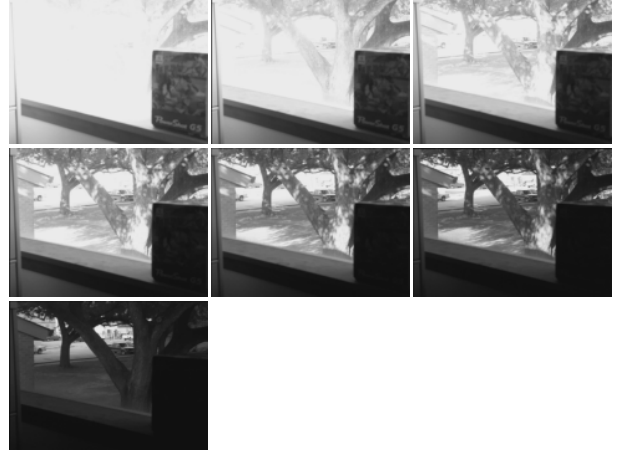
Fig. 2. Images of the same scene captured with a Canon G5 digital camera. The exposure times are 1/25, 1/50, 1/100, 1/200, 1/400, 1/800, and 1/1250 seconds. Original image size is 480 \times 640 .
