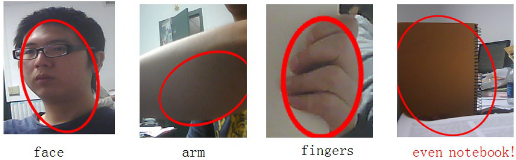
Figure 4: Detection Error Using CAMShift
