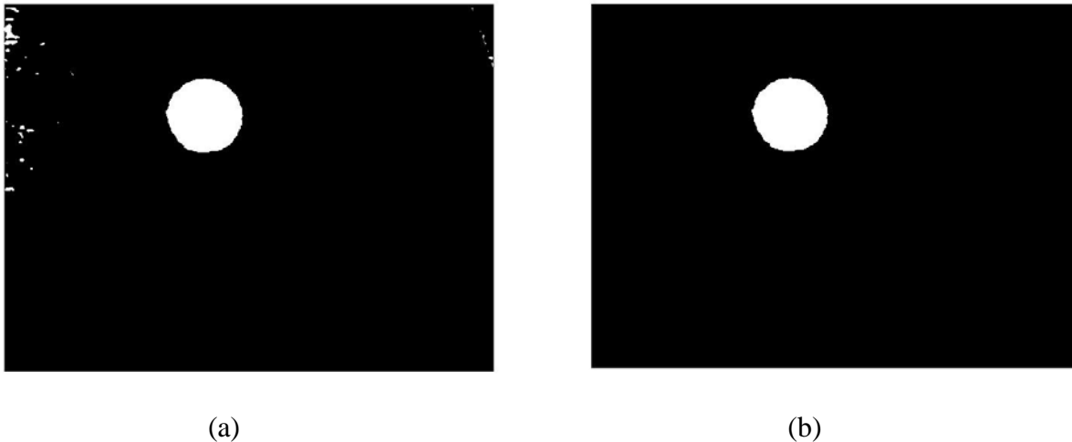
Figure 4. (a) Before removing the small areas, (b) after removing the small areas (less than 300 pixels)
