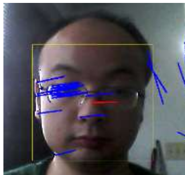
Figure 11 face tracking by optical flow
