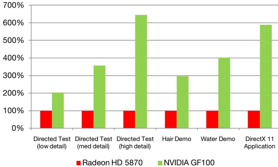
*The left three bars in the chart show tessellated geometry performance for three directed tests that focus exclusively on tessellation performance. As geometric complexity is increased, GF100's performance lead over the competition increases. The Hair and Water demos include both shading and compute operations in addition to geometry processing. The rightmost bar shows the performance of a tessellation state bucket (a set of draw calls from a frame) from a DirectX 11 application.*
