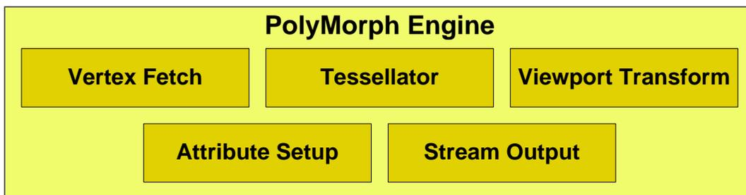
The first stage begins by fetching vertices from a global vertex buffer. Fetched vertices are sent to the SM for vertex shading and hull shading. In these two stages vertices are transformed from object space to world space, and parameters required for tessellation (such as tessellation factor) are calculated. The tessellation factors (or LODs) are sent to the Tessellator.
