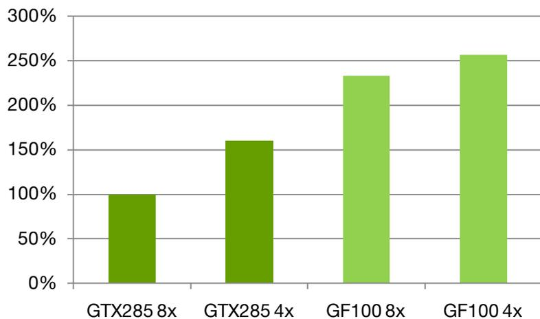
*Antialiasing performance, especially 8xMSAA, is significantly improved on GF100.*
