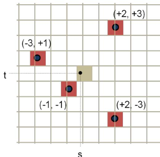
The soft shadows in 3DMark 2006 (left) are implemented through jittered sampling of a texture map (right). GF100 implements jittered sampling in hardware, delivering up to 2x the performance of GT200.
