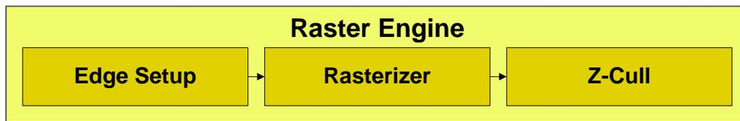
The Raster Engine is composed of three pipeline stages. In the edge setup stage, vertex positions are fetched and triangle edge equations are computed. Triangles not facing the screen are removed via back face culling. Each edge setup unit processes up to one point, line, or triangle per clock.
