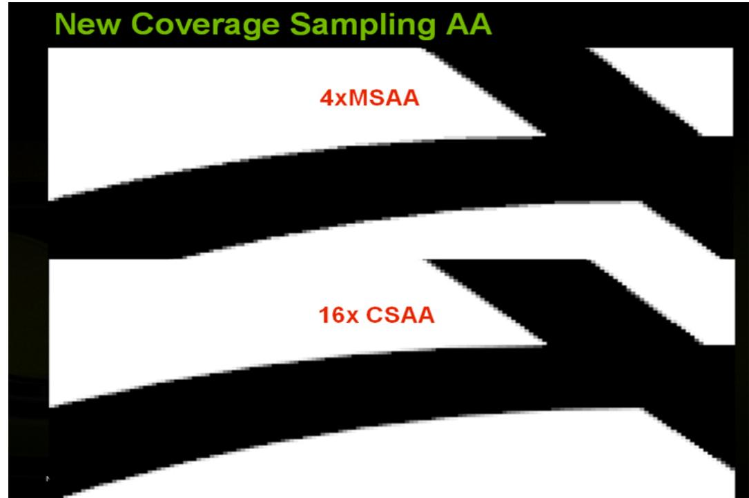
Figure 19. Coverage sampling antialiasing ( $4\times$  MSAA vs.  $16\times$  CSAA)
