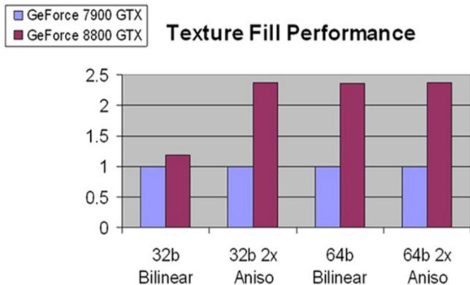
Figure 27. Texture fill performance of GeForce 8800 GTX
