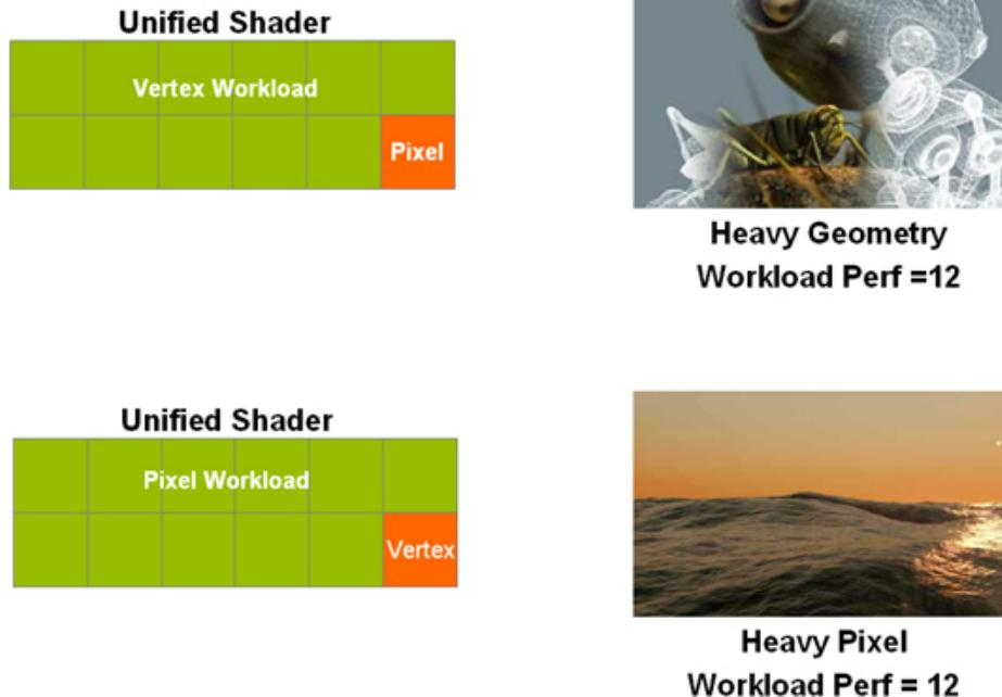
Figure 16. Unified shader performance characteristics
