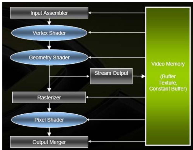
Figure 28. Direct3D 10 pipeline
