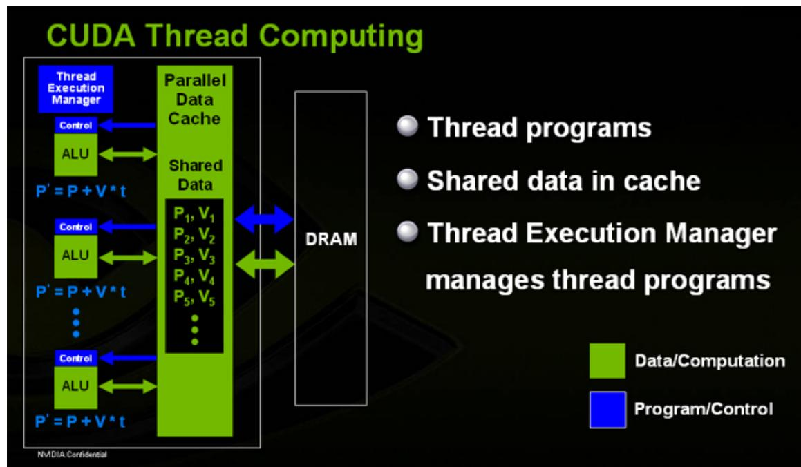
Figure 10. CUDA thread computing parallel data cache
