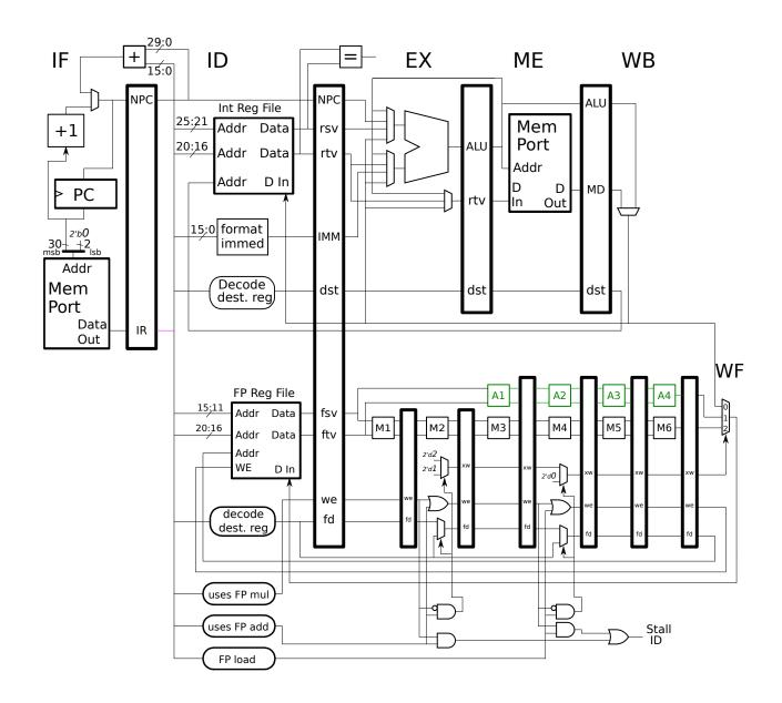
Functional Units and Pipelining > Unpipelined Units
