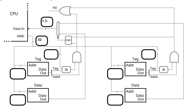
Complete the address bit categorization below. Label the sections appropriately. (Index, Offset, Tag.)
