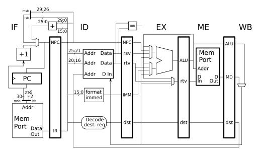
(a) Show the execution of the code below on the illustrated implementation up to the point where the first instruction, addi r2,r2,16, reaches WB in the second iteration.
