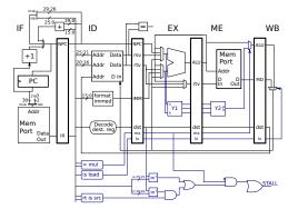
(a) Add hardware to bypass the product to the ALU and to the **rtv** mux when **b** is small. (There is a larger diagram on the next page.) The bypass should allow the first code fragment below to execute without a stall.
