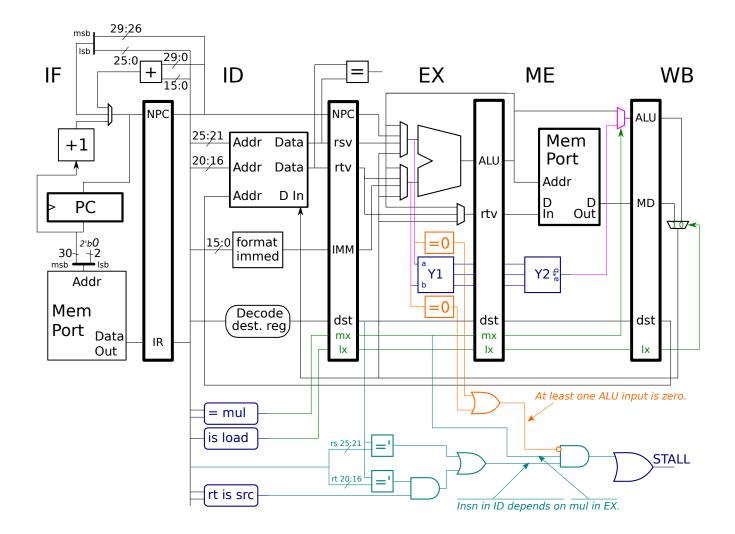
**Problem 2:** Though two stages (Y1 and Y2) may be necessary to compute the product of arbitrary 32-bit signed integers, there are special cases that can be computed in less time, for example when either operand is zero or one.
