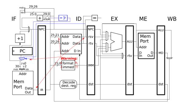
(a) The diagram shows a warning in red with lots of arrows and an explanation. Alas, the explanation is covered by the format immed box. Assume that the hardware for  $\Im r$  is correct. Then what can the warning be about?
