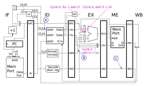
(a) The illustration has several circled letters pointing to wires. In the diagram below show the values on those wires on each cycle the value is used.
