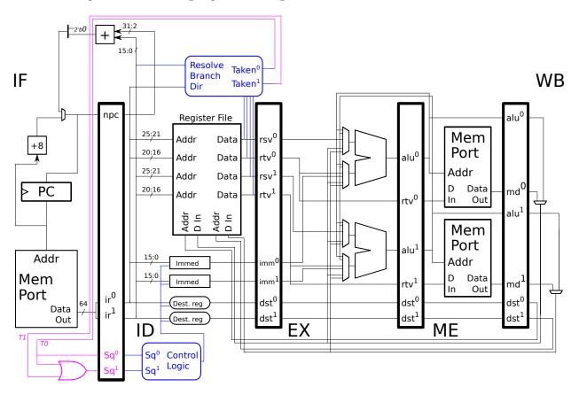
(a) When a branch is taken we may need to squash one or two instructions (the number of instructions to squash depends on the whether the branch is in slot 0 or slot 1). Design logic to set the Sq0 and Sq1 inputs so that appropriate instructions are squashed. It will be very helpful to draw pipeline execution diagrams showing a taken branch in slot 0 and slot 1.
