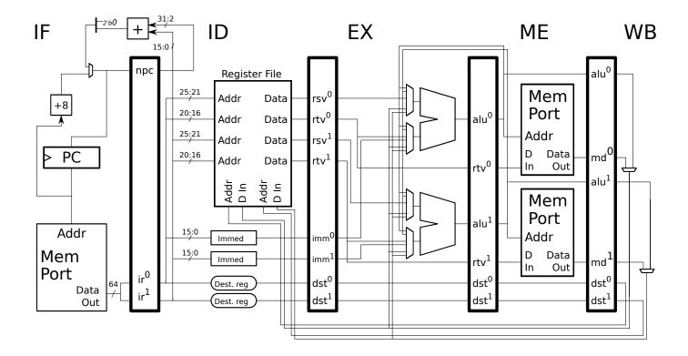
Problem 2: (10 pts) Appearing below is the execution of a bit more than two iterations of a loop on the illustrated MIPS implementation. The execution shows the use of a two-stage FP compare unit, C1-C2, by the c.lt.s instruction, but the unit isn't shown.
