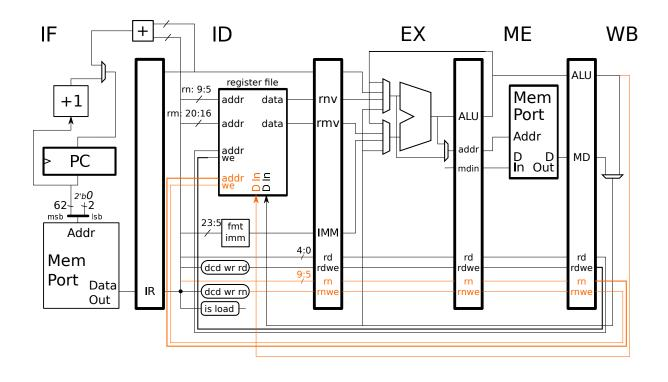
0 rd rn : Writes rd and rn. Post-index ldr x1, [x2], #8 0 x1 = Mem[x2]; x2 = x2 + 80 rd : Writes rd and rn. Pre-index rn ldr x1, [x2, #8]!  $0 x^2 = x^2 + 8; x^1 = Mem[x^2];$ 0 rd rnrmstr x1, [x2, x3] 0 Mem[x2+x3] = x1
