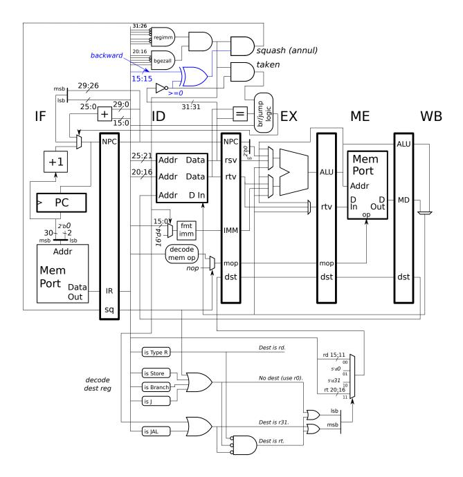
Solution appears above. Whether the branch target is before or after the branch can be determined by looking at the sign bit of the immediate value, which is bit 15 of ID.IR and is labeled **backward** in the diagram above. If that bit is
